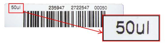
When *loading manually* and there is *no library available* for distinguishing the different tip types used, *visual inspection* of the barcode label is the only option. This is the case for Slim Tips, 10-300µl used in combination with CO-RE Tips, 10-1000µl.
