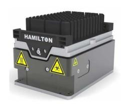
The HHS can be heated to temperatures up to 105°C. The temperature is constantly measured by two sensors, one located in the middle and one at the edge of the adapter plate.
