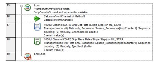
10. In the CO-RE gripper "Get Plate" Command, set the "FrontChannel" Variable.
