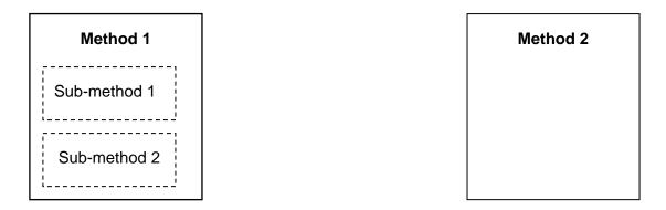
A **sub-method library** contains an independent sub-method that may be used in several independent methods. To make use of the advantages of sub-methods, the functions of the "**Sub-method**" Library has to be included in a method.
