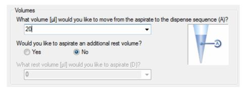
7. In this step, select a tip sequence (e.g. "ML\_STAR.MIStar300ulStandardVolumeTip") from the drop-down field or "Drag and Drop" it from the Deck Layout. The tip handling chosen here is to take new tips for each sample.
