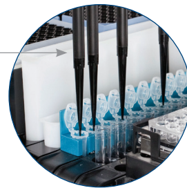
Pipet known standards to determine pressure curves
