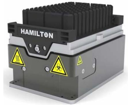
The HHS can be heated to temperatures up to 105°C. The temperature is constantly measured by two sensors, one located in the middle and one at the edge of the adapter plate.
