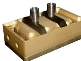
COREGripTool OnWaste 5ml uses a holder for the paddles mounted on top of the waste block. This is a holder that is capable to hold both 1000µl-pipetting channel and 5ml-pipetting channel paddles. Using this labware will create the default sequence for 5ml-pipetting channel paddles.
