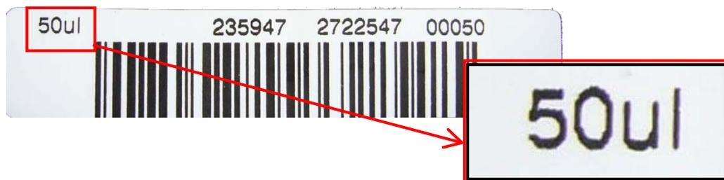
When **loading manually** and there is **no library available** for distinguishing the different tip types used, **visual inspection** of the barcode label is the only option. This is the case for Slim Tips, 10-300µl used in combination with CO-RE Tips, 10-1000µl.
