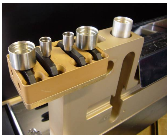
CO-RE Grippers mounted on waste block: 1000µl-Pipetting Channels (inner positions) and 5ml-Pipetting Channels (outer positions)
