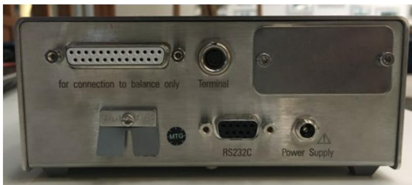
Figure 4-3: Viewing the ports on the control box
