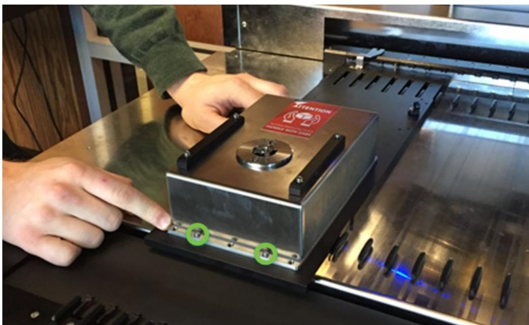
Figure 4–1: Placing the balance on a carrier base
