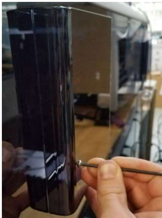
Figure 2-21: Securing slot covers to prevent UV exposure out the rear of the instrument
