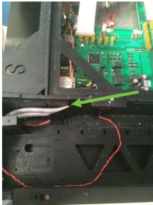
Figure 2-8: Route the sensor cable connectors
