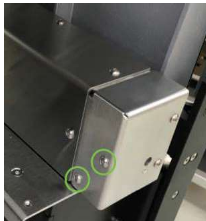
Figure A-12: Attaching the end cap cover
