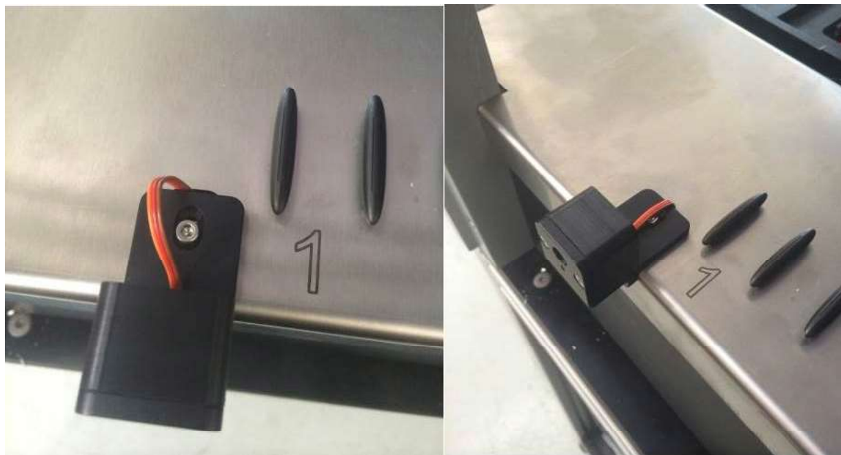
Figure 2-15: Attaching the sensor
