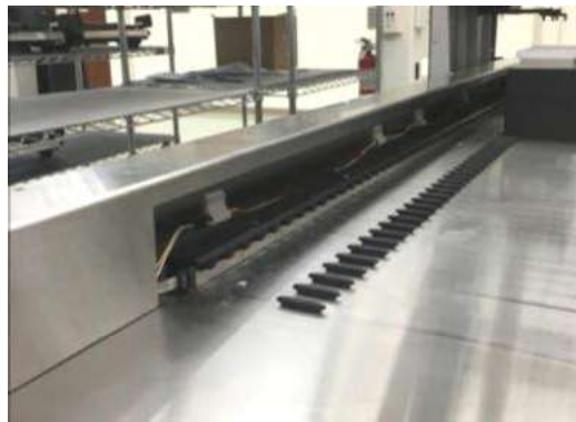
Figure A-11: Installing the back cover
