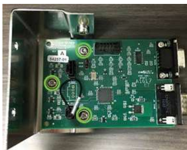
Figure A-5: Detaching the PCB from the old cap
