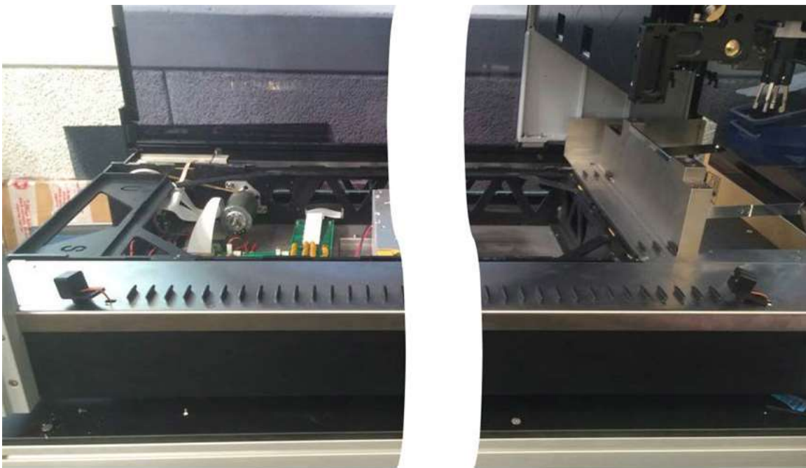
Figure 2-14: Installing the front deck sections
