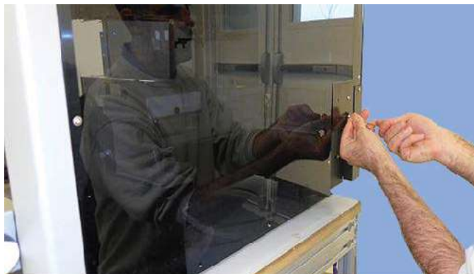
Figure 2-26: Securing the right side tube routing cover
