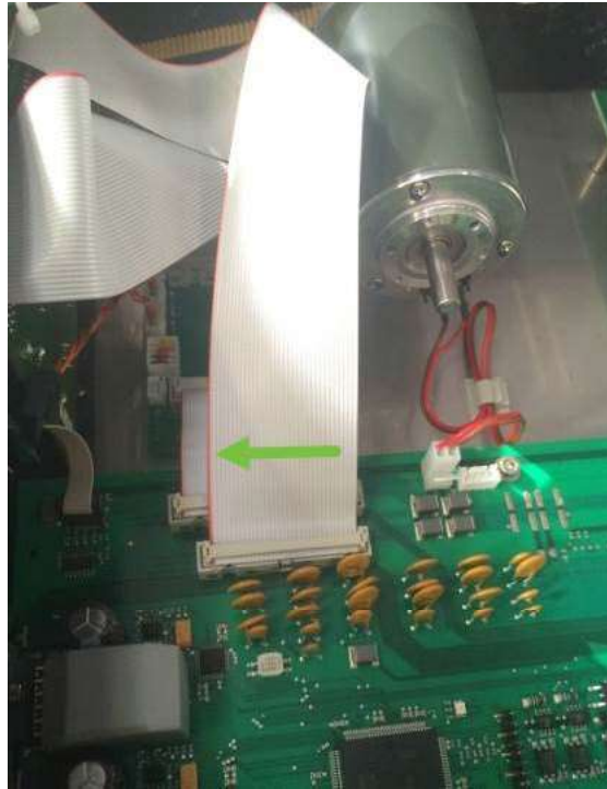
Figure 2-11: Reconnecting the periphery ribbon cable
