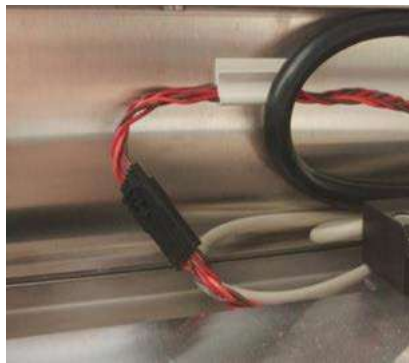
Figure A-7: Connecting the end cap cable
