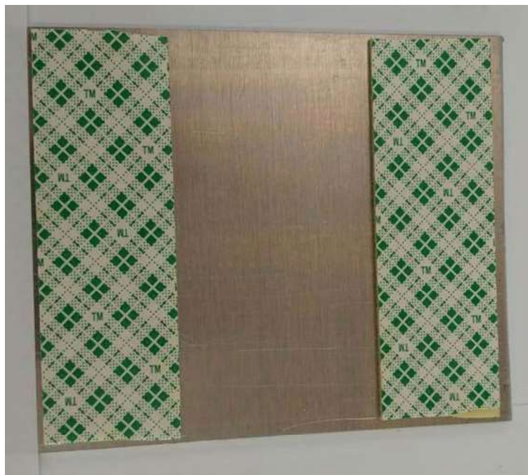
Figure 2-5: Applying double-sided tape to the back of the PCB mount
