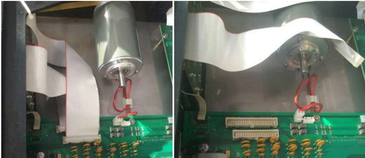
Figure 2-7: Disconnecting the ribbon cables from the dual processor board
