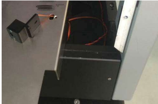
Figure 2-13: Mounting sensors on their brackets
