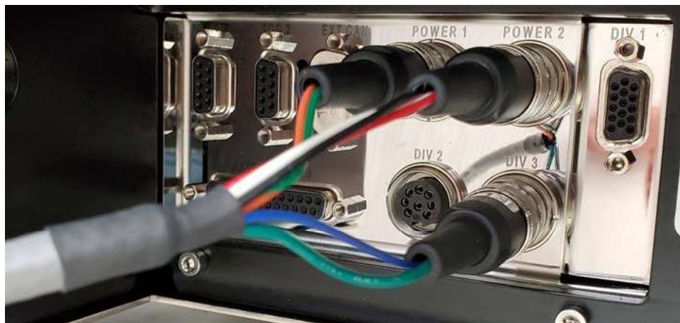
Figure 2-30: Power (POWER 1 and 2) and communication (DIV3) ports
