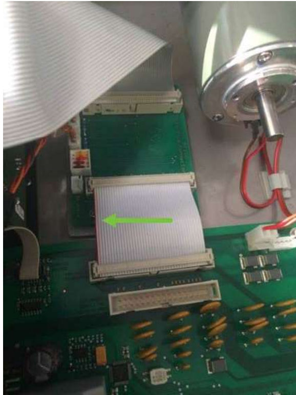
Figure 2-10: Attaching the flow connector board
