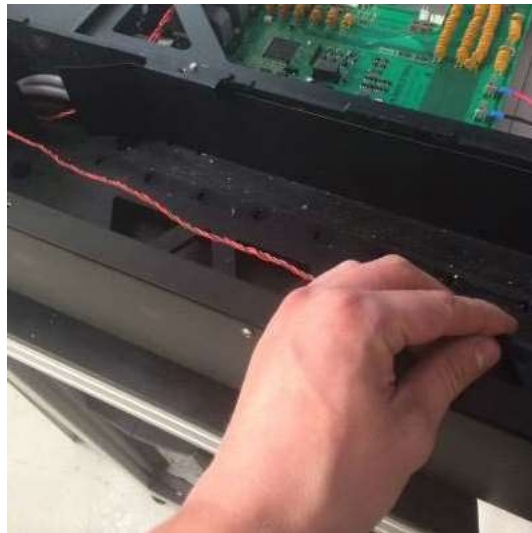
Figure 2-12: Routing sensor cables
